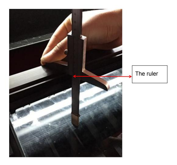
2. If the distance is not same, please adjust the nuts in the machine. It can keep the platform balance.
