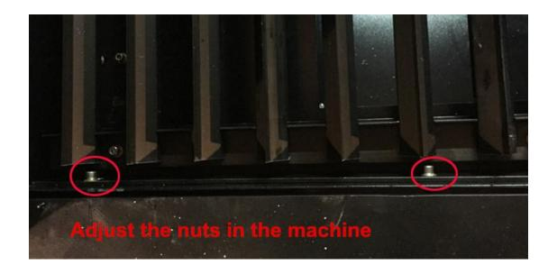
**Note:** The deviation of measurement from the guide rail to the glass can't exceed 4 mm.
